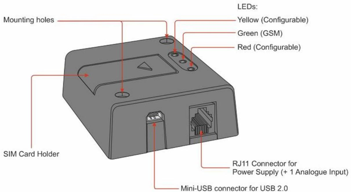
Figure 1: Connector on rear side of the Terminal
