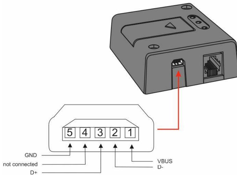
**Figure 5: Mini USB Type A/B connector for HT910 E and HT910 E USB Powered**
