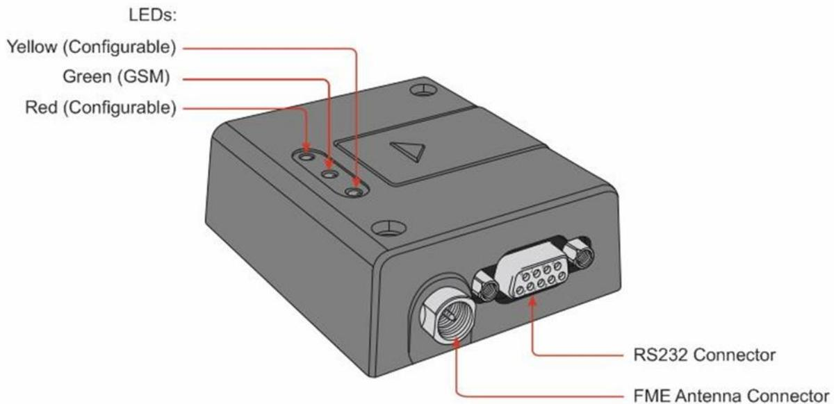
**Figure 2: Connectors on front side of the Terminal**
