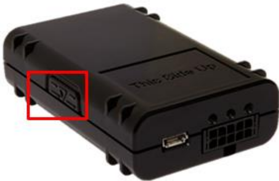
Picture 6: The button to open the SBC AVL 4G Housing
