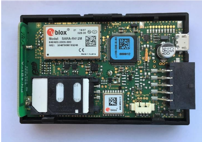
Picture 9: Where to insert the SIM Card
