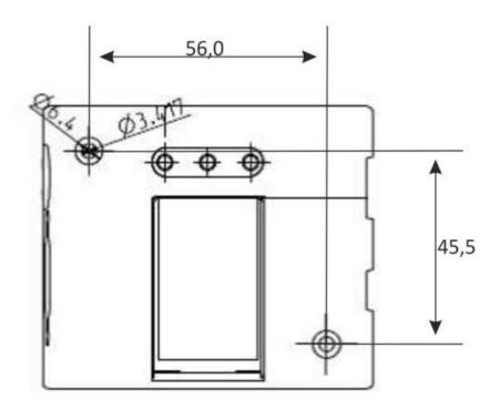
Figure 3: Drawing of the Terminal's Housing
