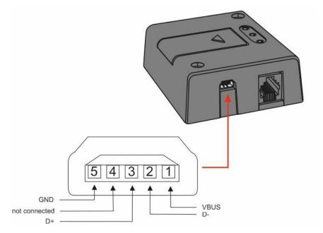
Figure 5: Mini USB Type A/B connector for HT910 E and HT910 E USB Powered
