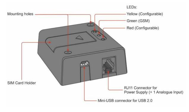
Figure 1: Connector on rear side of the Terminal
