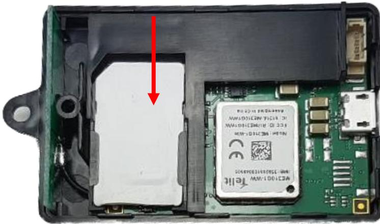
Figure 2: How to insert the SIM Card
