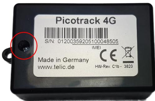
Figure 1: How to open the device
